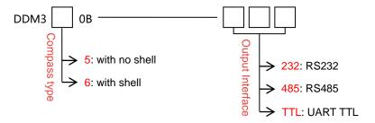
Eg.: DDM360B-232: 3D compass with shell, RS232 output
